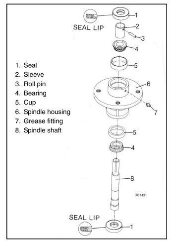
Figure 13. Blade Spindle Assembly
